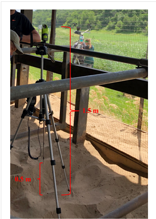
FIGURE 1 Photo of how air speed was measured in a stall (1 min per location). To obtain air speeds at cow standing (1.5 m) and resting (0.5) heights, a propellor anemometer on a rotating vane mount and a hot wire anemometer were used, respectively. The two devices were mounted on the same tripod, as demonstrated in the photo, and placed in the middle of the stall with the notch on the end of the hot-wire anemometer facing toward the direction of oncoming air flow.
