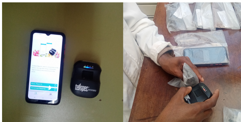
FIGURE 2 Telspec handheld NIR spectrometer (left) and demonstration of how each sample was scanned (right).
