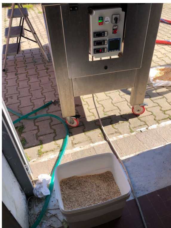
FIGURE 1 Chestnut wood next to the HC-based reactor prior to undergoing hydrodynamic cavitation.
