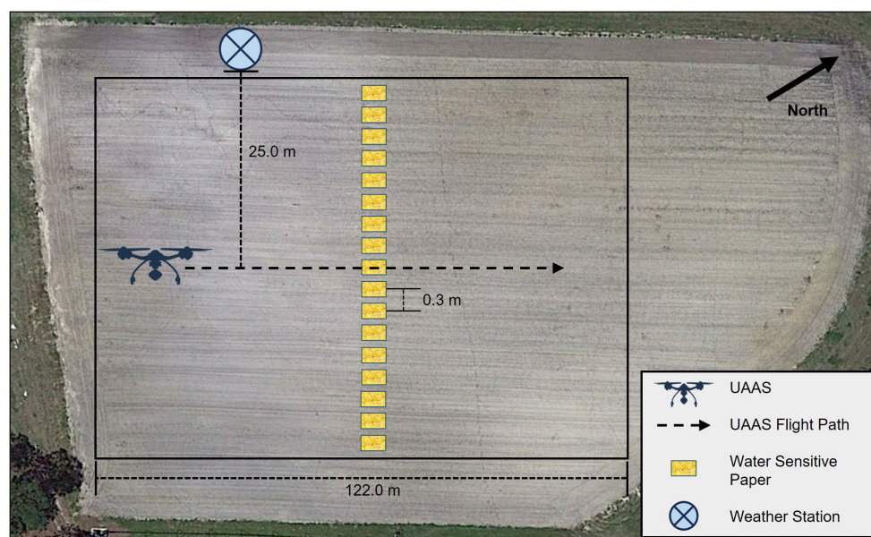
FIGURE 3 Illustration of the data collection setup in the test area used for collecting spray deposition data for each UAAS.
