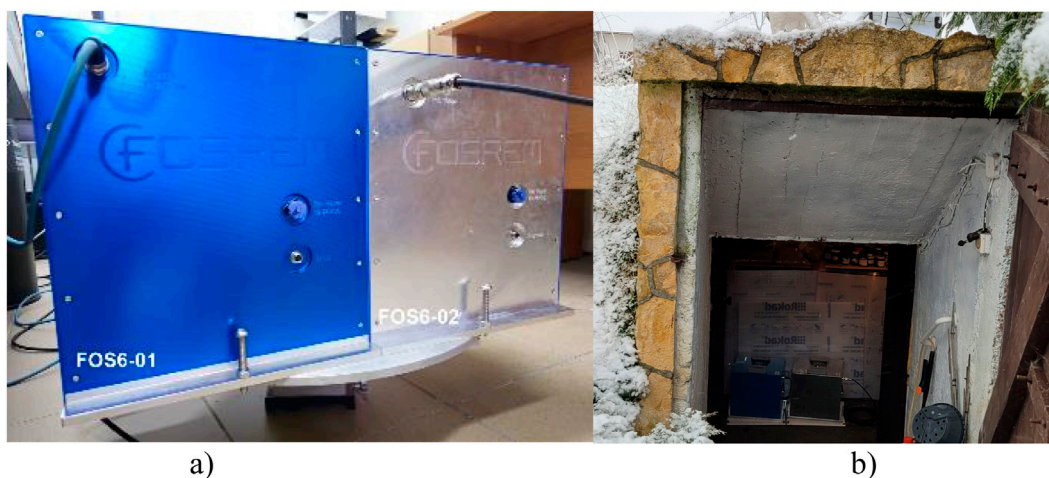
FIGURE 5 Two FORSs type FOS6 situated on a leveled board: (A) FOS6-01 and FOS6-02 in the MUT laboratory on the rotary table. (B) FOS6-01 and FOS6-04 in a basement about 1.5 m below ground level in the Kampinos Nature Park, Poland.
