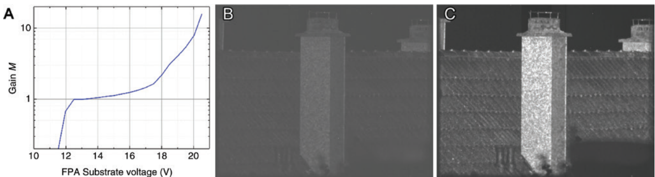
Figure 2: Camera-level gain curve of a 640 \times 512 InGaAs-APD camera operated at 140 K (A), GV images taken with FPA substrate voltages of 13 V and 19.7 V corresponding to gain values M = 1 (B) and M = 6 (C), respectively.
