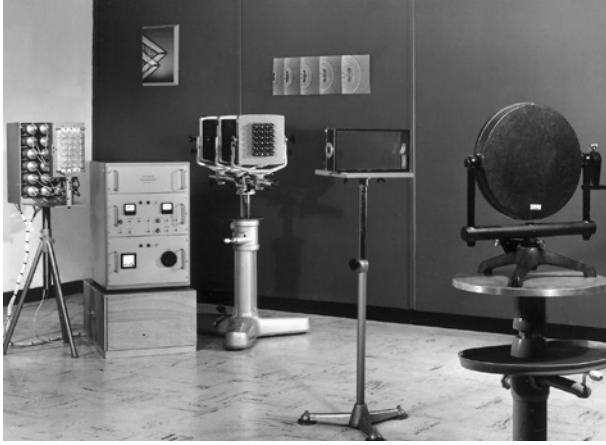
Figure 1: Cranz-Schardin chronolens with spark illumination. This camera contributed to spectacular progress in the comprehension of aerodynamics and gas physics.
