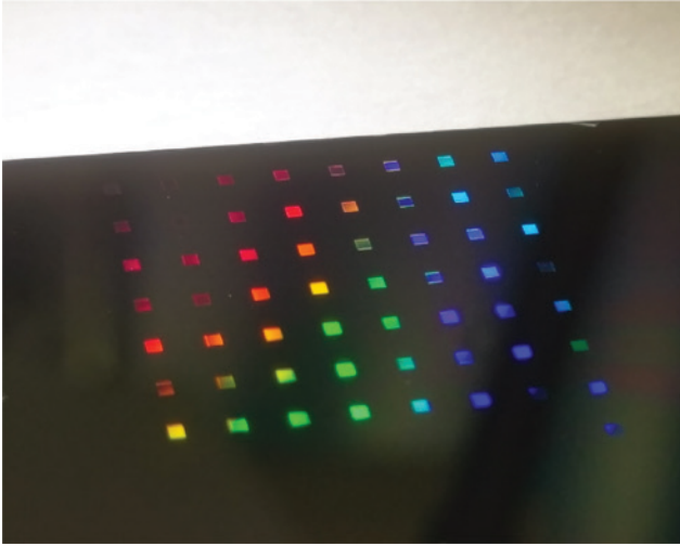
Figure 7: Photograph of an 8 \times 8 array of three-dimensional PMMA patterns, each (0.575 \text{ mm})^2 in area, obtained by the Talbot effect when illuminated to unpolarized white light. Owing to the periodicity of the structures, the element shows optically dispersive behavior in the visible.
