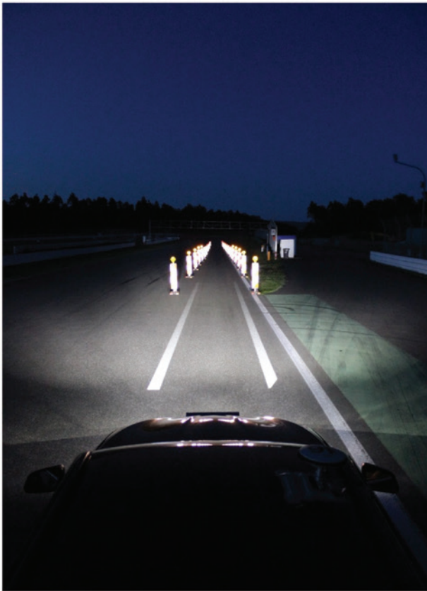
Figure 8: A BMW 5 series equipped with a projector in the radiator grill. Before entering the narrow path, two parallel lines in positive contrast appear and show the car width.
