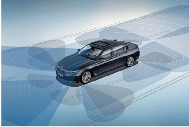
Figure 1: Exemplary presentation of the already implemented sensor systems in nowadays cars.
