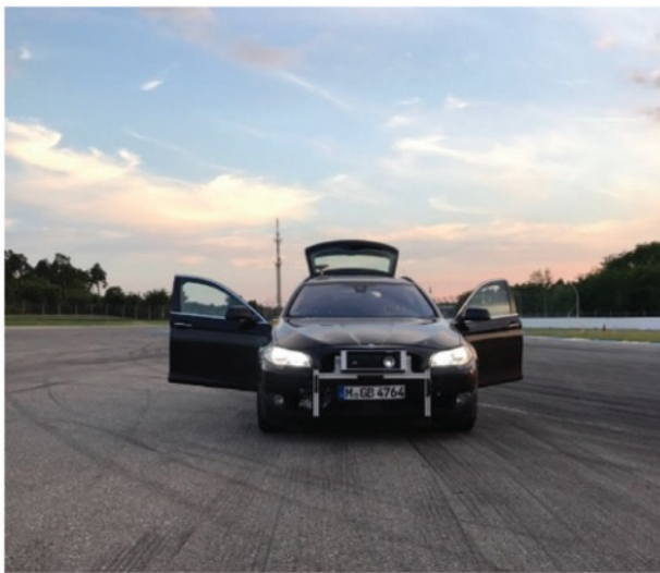
Figure 10: BMW5 series with an external projector implemented in the car's radiator grill for the projection of positive contrasted symbols on top of the car's LED low beam.
