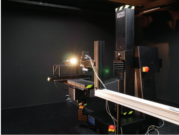
Figure 7: Goniophotometer with video photometer and spectrometer.
