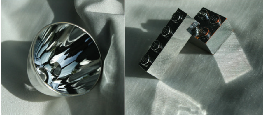
Figure 1: Left: An aluminum-coated reflector on a lathe-processed aluminum substrate produces a simple paraboloid for flashlight applications with a specular surface. The base of the reflector is pressed against the ‘pill,’ its vertex hole centers the reflector on a specific type of LED. Right: Aluminum-coated plastic parts (play bricks) to illustrate the conformal coating with metal on plastic and to show the impact of a small surface contour deviation on the ‘beam pattern’ of reflected light. Sunlight is incident from the right in this photograph. The reflection of sunlight off the long brick on the bottom left shows distortions and artifacts caused by the surface contour which is not flat; the reflection by the right brick shows a smooth light distribution: its surface is flat.
