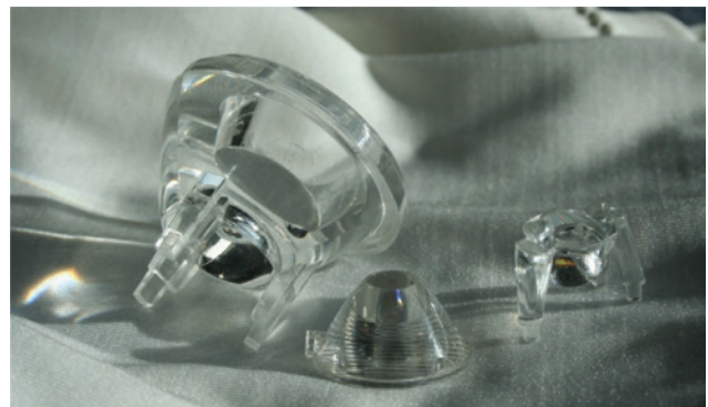
Figure 2: TIR reflector examples: Collimator LED lenses are hybrid devices that use a front lens shape and a side reflector to direct light. The smooth paraboloid shape is the (freeform) TIR reflector of these components. These samples are made of PMMA through injection molding.
