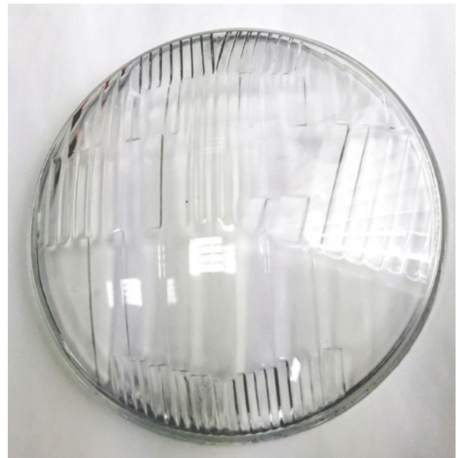
Figure 5: Classic headlight lens made of glass for low- and high-beam creation, showing the traditional shard grid where each facet serves a specific purpose; contrast-enhanced black and white photograph. Each shard is nowadays a single freeform surface facet to be designed and calculated individually with respect to the other facets and their contribution to the combined beam pattern. This original sample was designed for a dual-filament bulb.
