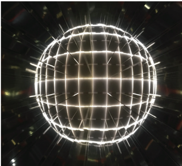
Figure 16: Look into a hollow tapered rod of square cross section. The rod was standing on a table with the rim of the smaller bottom face illuminated from the side (Photo courtesy by Markus Stange, OSRAM).
