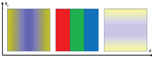
Figure 9: Schematic phase space diagrams of various LEDs. Left: White LED (blue chip embedded in phosphor matrix) as shown in Figure 8, middle, with its spatial color distribution. Center: Multi color LED package with adjacent red, green and blue chips. Right: Thin film white LED (blue thin film, surface emitting chip covered with thin phosphor layer), with its spatial homogeneity and its typical color over angle distribution.
