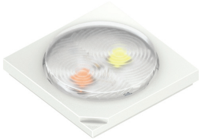
Figure 7: A small cell phone flash LED with a cold white (top right) and a warm white (bottom left) LED chip, with identical Fresnel lenses for each LED. Perfect color mixing of these two sources is achieved, except at very close distances which are not relevant for this application. (Image courtesy OSRAM Opto Semiconductors GmbH.).
