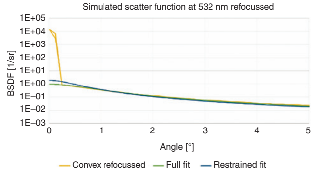
Figure 14: Fit to measured data for all three parameters and with fixed L and S values.
