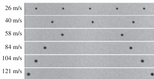
Figure 11: Higher-velocity droplets arrive at the target location with greater spacing.
