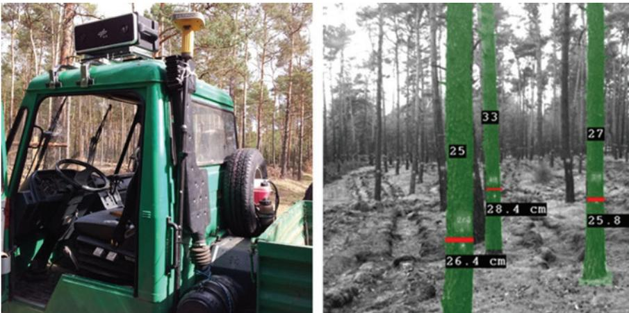
**Figure 8:** IPS outdoor system mounted on a forestry vehicle (left), automatically identified, labeled, and localized single trees based on IPS information (right).
