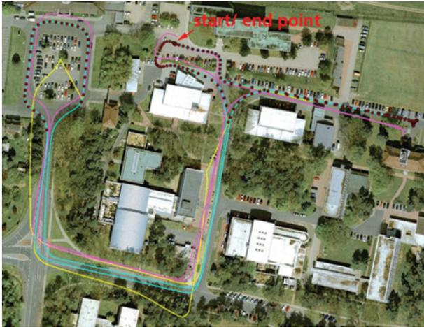
**Figure 5:** Comparison of the accuracy of different localization technologies in an outdoor scenario (IPS mounted on a vehicle, closed loop). DGPS reference points (red dots), IMU trajectory, fused with GPS if available (yellow, covered at some places with GPS measurements), visual-odometry-only trajectory (magenta), visual-aided IMU trajectory, fused with GPS if available (cyan).
