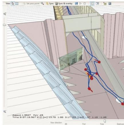
**Figure 6:** Ship inspection as an example for an IPS application, helmet-based system in operation (left), IPS trajectory and inspection photograph laid over a CAD model of a ship, visualized in ShipManager Hull © (right).
