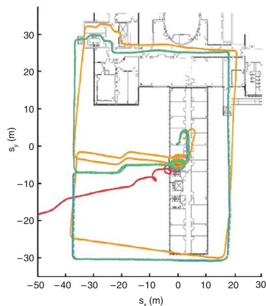
**Figure 4:** Comparison of the accuracy of different localization technologies in an indoor scenario (hand-held IPS). Reference trajectory (green), IMU-only trajectory (red), visual-odometry-only trajectory (yellow), and visual aided IMU trajectory (blue).
