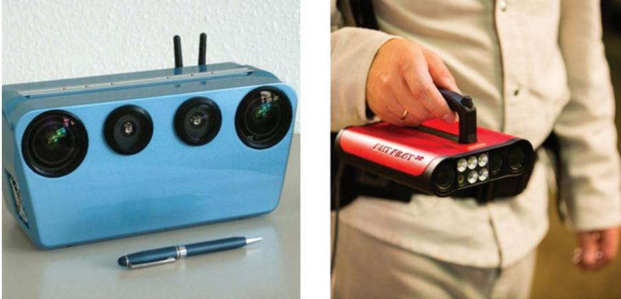
**Figure 2:** Integrated positioning system (IPS). Functional demonstrator (left), commercial prototype (right).
