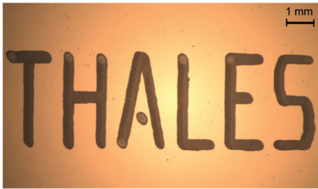
Figure 8: The 2D laser marking at 3.47 \mu\text{m} on a pyroelectric camera damage test plate.
