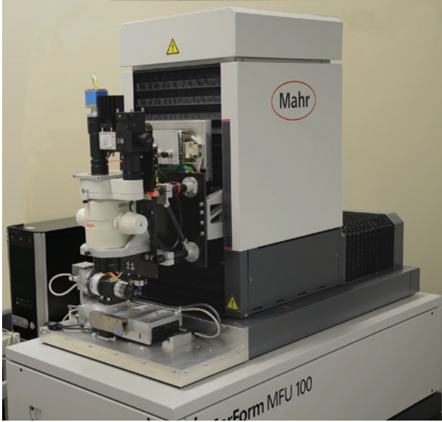
Figure 3: Exemplary picture of a multi-scale inspection system equipped with a zoomable fringe projection microscope and a chromatic confocal point sensor.
