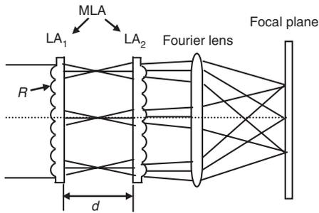
Figure 25: Structure of imaging homogenizer.
