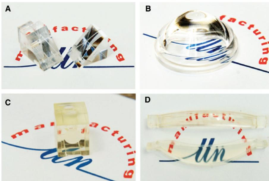
**Figure 24:** Imaging plastic optics (the maximum side length of the reference logo 55 mm): (A) prism for a beam splitter in augmented reality (AR) systems, (B) biconvex lens, (C) light collimator lenses, (D) f- $\theta$  scan lenses with freeform optical surfaces.
