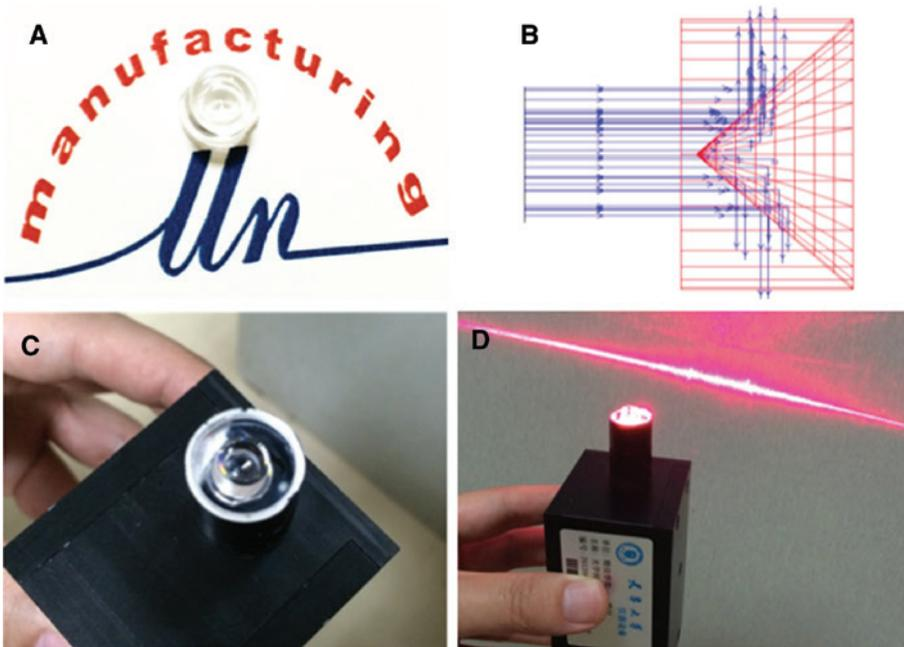
Figure 28: Laser total reflection system: (A) micro injection molded total reflection system, (B) schematic of optical path, (C) lens assembled with a laser beam, (D) laser project from sidewall of lens.
