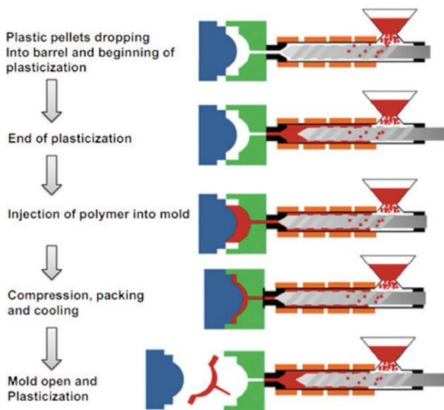
Figure 14: Simplified schematic of injection compression molding process.
