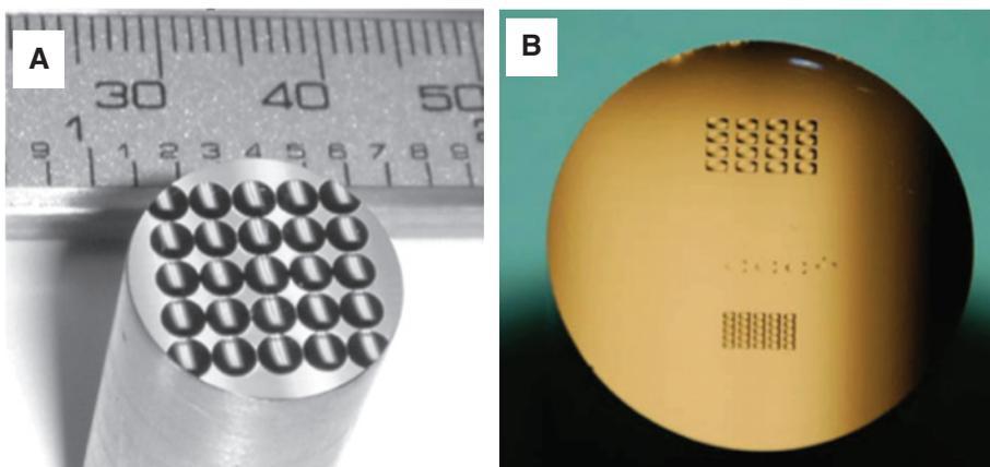
**Figure 5:** Freeform microlens array (A) and Alvarez lens array [19] (B) machined by SSS ultra-precision turning process [20].
