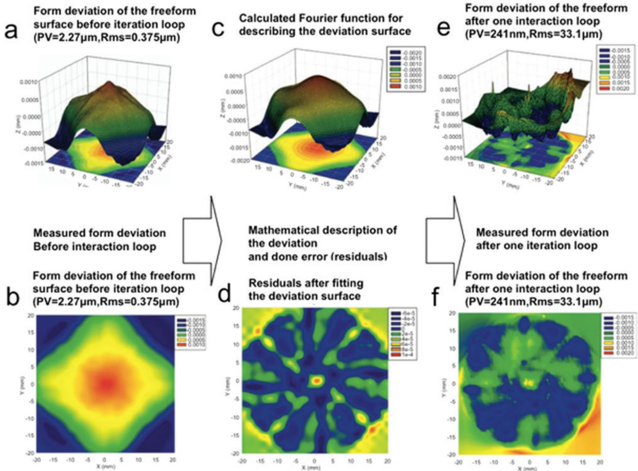
**Figure 11:** Details of the iteration loop for machining a high precision freeform surface on the mold: (A) Surface deviation before iteration loop, 3D view; (B) surface deviation before iteration loop, top view; (C) Fitted Fourier function as error description of the surface deviation; (D) error between fitted deviation and found mathematical description; (E) surface deviation after one iteration loop, 3D view; (F) surface deviation after one iteration loop, top view [21].
