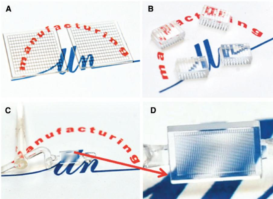
Figure 27: Compound eye lens arrays (the maximum side length of the reference logo 55 mm): (A) plano-aspheric lens arrays, (B) double sided compound lens arrays, (C) double side MLSs, (D) enlarged view of a microlens arrays.
