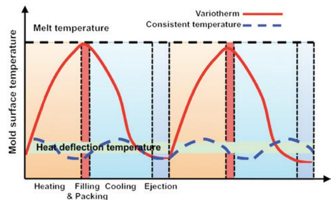
**Figure 16:** Under variotherm mold temperature control system, mold temperature increases to/over material’s glass transition temperature to reduce material viscosity and flow resistance, to diminish welding lines and help surface replication. In cooling stage, mold temperature is reduced to material’s deflection temperature in order to eject part out safely [49].
