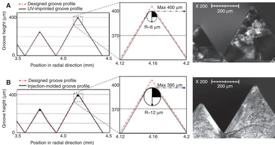
**Figure 23:** Designed and measured profile and cross-sectional images of (A) a UV-imprinted MFL with a GPR of 6 μm and (B) an injection-molded MFL with a GPR of 12 μm [63].
