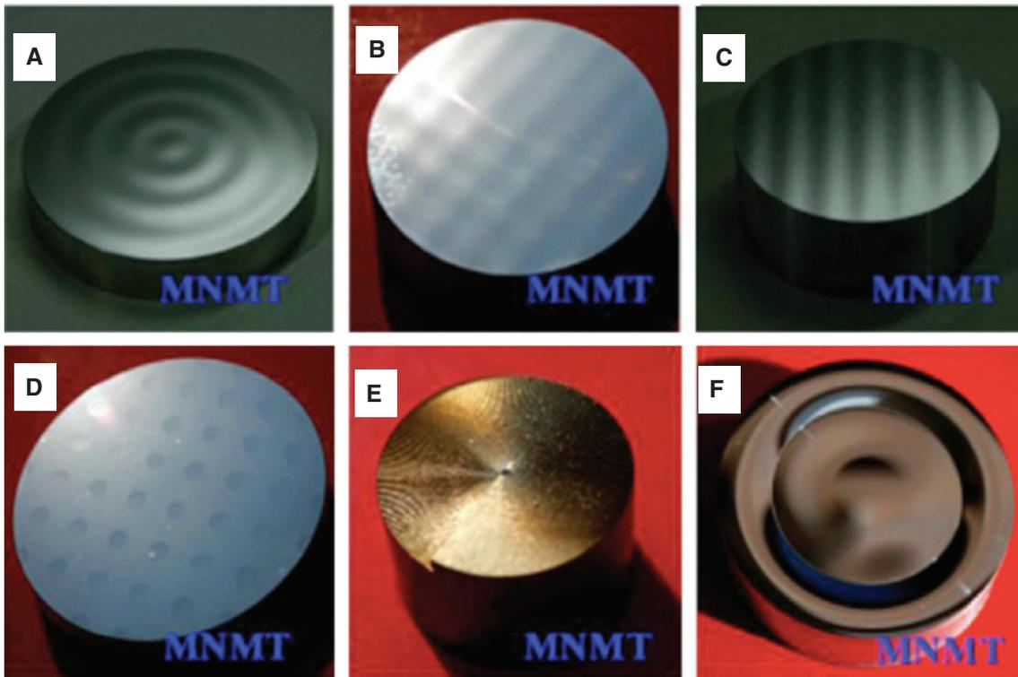
**Figure 4:** Typical freeform optics fabricated by the cylindrical machining method: (A) water-drop freeform, (B) sinusoidal freeform, (C) cylindrical freeform, (D) aspheric lens arrays, (E) spiral freeform, (F) integrated freeform.
