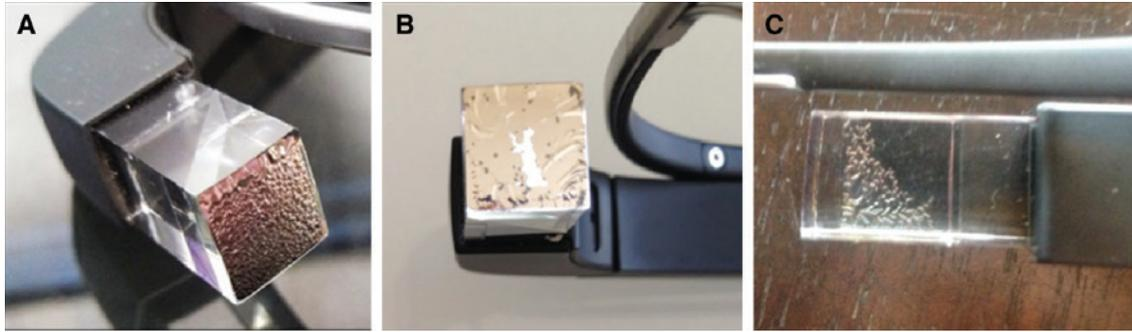
**Figure 29:** The failure of Google glasses in service: (A) bubbled surface formed on a concave reflector in a humid and hot weather [66], (B) delamination of coatings of concave reflector [67], and (C) breakage between 6-month use [68].
