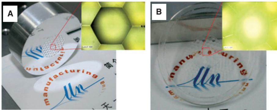
**Figure 7:** Optical device of the compound eye: (A) fabricated mold using SSS, (B) compound eye lens fabricated by microinjection molding [22].
