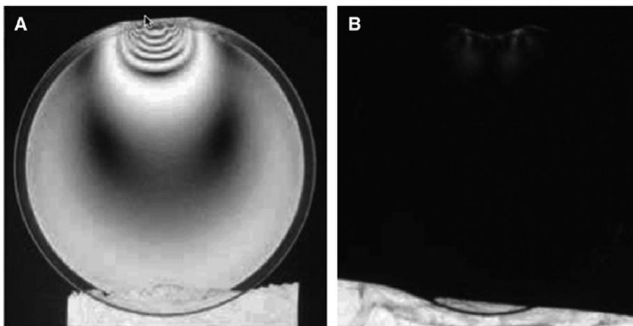
Figure 20: Distribution of residual birefringence of plano-convex lens with a diameter of 50 mm and a thickness of 2 mm: (A) directly injection molded part, (B) part annealed at 153°C for 8 h [34].
