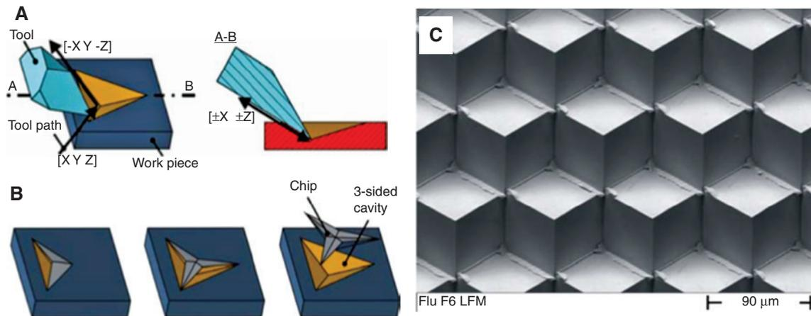
**Figure 10:** Diamond micro chiseling process for manufacturing cubic hexagon retro-reflector arrays: (A) principle of diamond micro chiseling, (B) cubic hexagon retro-reflector arrays [28], (C) the diamond micro chiseling machined cubic array with an individual circumference diameter of 100  $\mu\text{m}$  on an electroless nickel substrate with intruding edges caused by interactions of set-up accuracy, non-ideal tool geometry and plastic material behavior.
