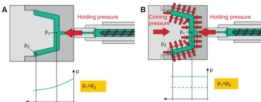
**Figure 13:** Schematic of injection molding and injection compression molding: (A) pressure distribution of conventional injection molding is related to part geometry and location of injection gate, (B) injection compression molding has more uniform pressure by adding a compression operation of a mold core [35].
