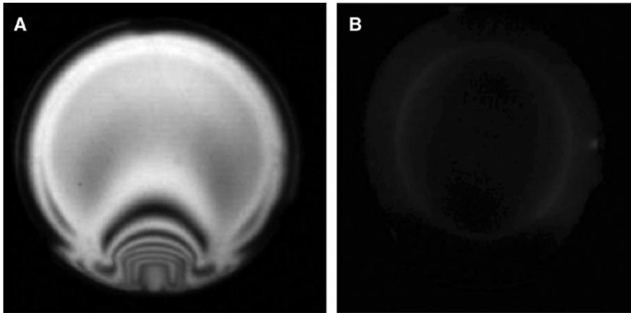
**Figure 21:** Distribution of residual birefringence: (A) preform with PV  $15.31 \mu\text{m}$ , RMS  $3.73 \mu\text{m}$ , (B) compression molding assisted annealing gives PV  $0.693 \mu\text{m}$  and RMS  $0.16 \mu\text{m}$  [60].
