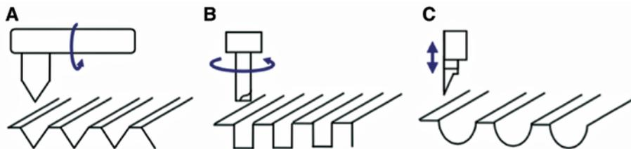
**Figure 9:** Selection of ultra-precision machining to produce 3D-microstructured surfaces: (A) raster milling, (B) end milling, and (C) FTS machining [27].
