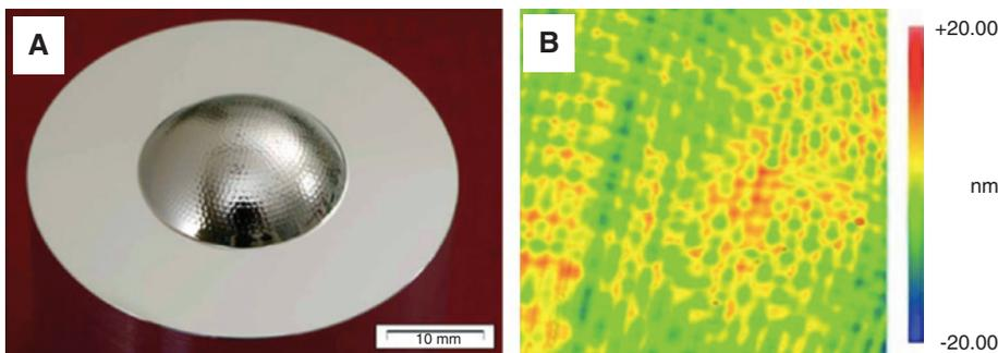
**Figure 8:** A finished freeform microlens array mold insert containing 1219 single spherical lens lets (A) with clear aperture of the lens area is 19 mm and the outside diameter of the substrate is 40 mm and topography of a single lens surface (B) [25].
