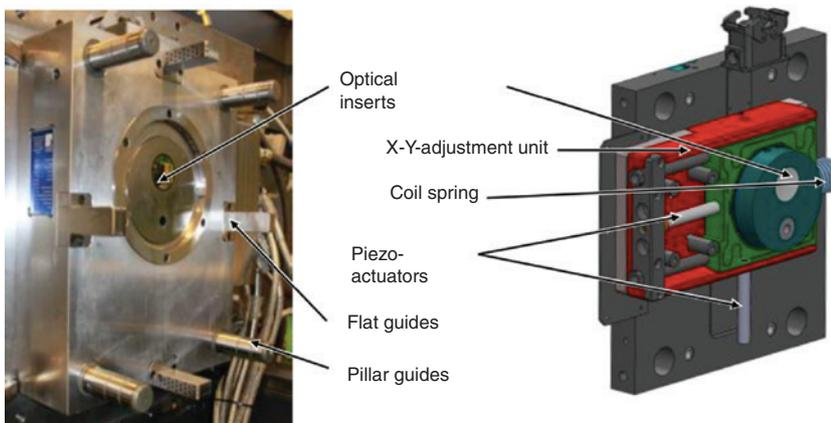
**Figure 12:** Fixed mold half with integrated adjustment unit using piezoelectric actuator [30].
