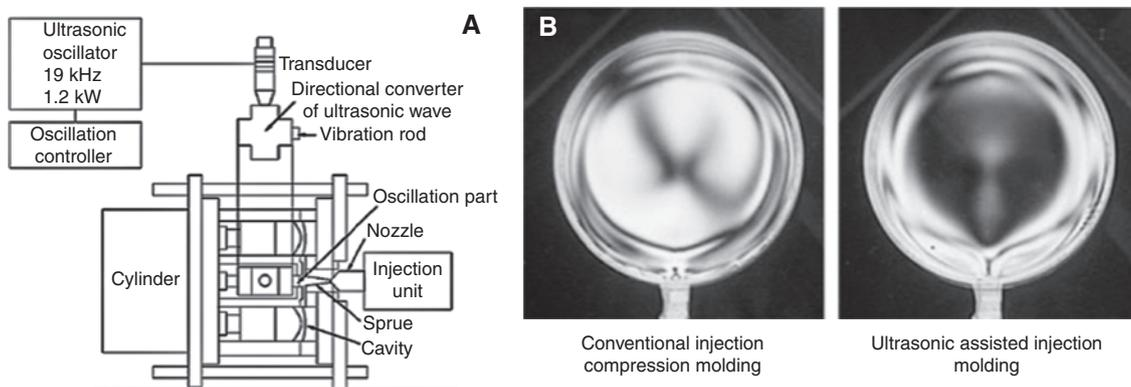
**Figure 18:** Schematic drawing of ultrasonic assisted injection molding system (A) and comparison of residual stress of conventional injection molded part and ultrasonic assisted injection molded part [57].
