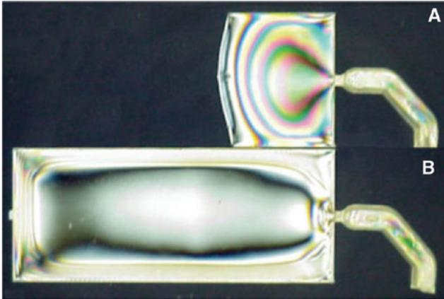
**Figure 17:** Effect of conventional injection molding (A) and variotherm assisted injection molding (B) on flow length and birefringence of 0.5-mm-thick PC [50], it can be seen that variotherm significantly increases flow length and decreases residual stress.
