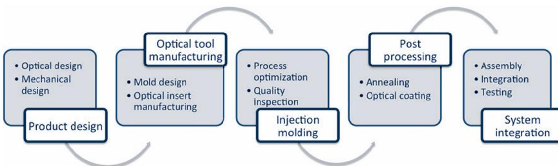
Figure 1: Process chains for manufacturing plastic optics.
