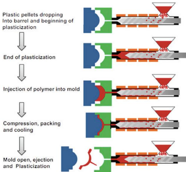
**Figure 2:** Simplified schematic of injection molding process.
