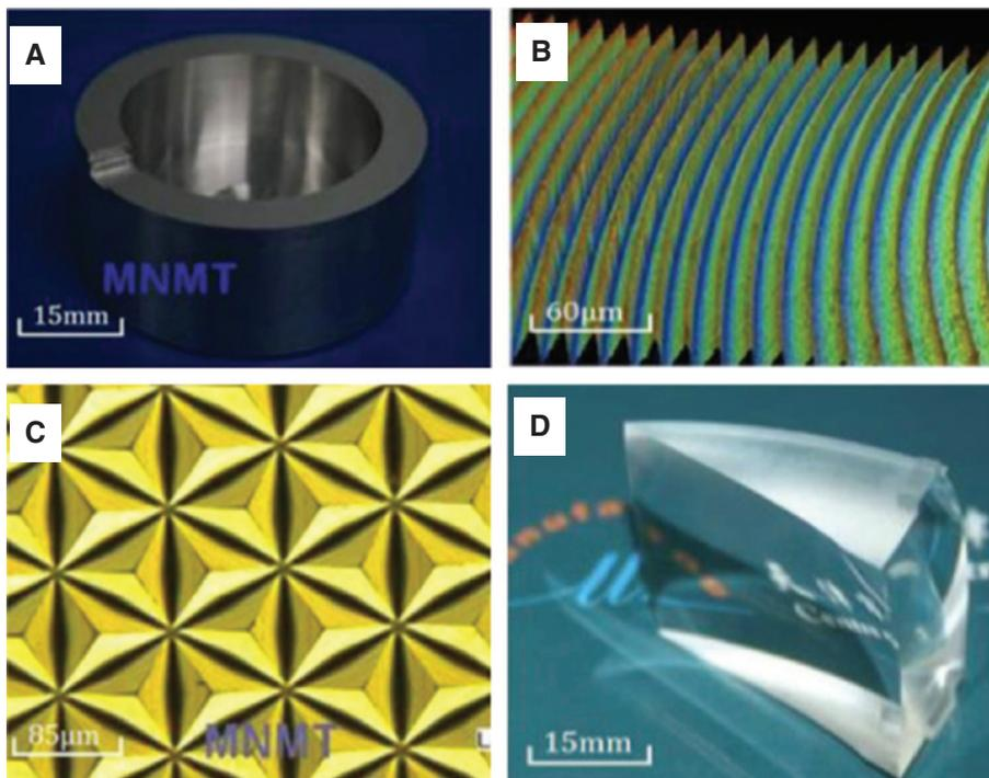
**Figure 3:** Freeform surfaces: (A) continuous smooth surfaces modeled using a mathematic formula and CAD software, such as spiral mirrors applied to the femto-second (fs) laser scanning; (B) a Fresnel lens with discontinuous surfaces include steps or facets; (C) structured surfaces, which are the arrays of structure for specific function, therefore called functional surfaces; (D) an optical freeform prism with multiple surfaces on a single substrate [5].
