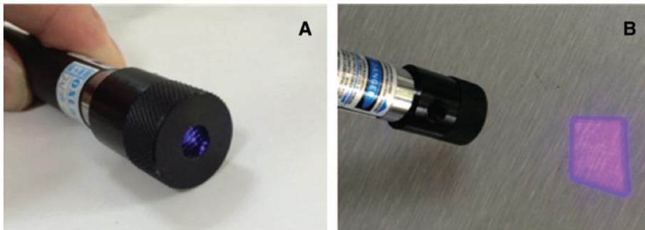
Figure 26: Double side MLAs for uniform illumination: (A) double-sided compound lens arrays assembly into a laser pointer, (B) a laser beam is uniformly projected on to a wall.
