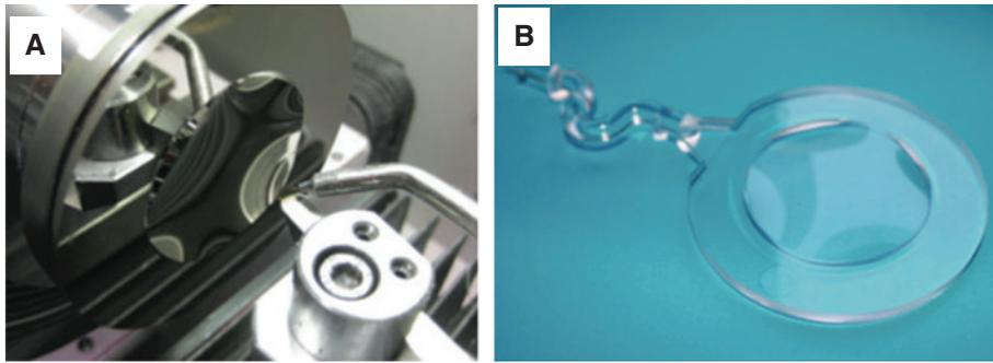
**Figure 6:** Freeform tool insert positioned at the vacuum chuck on the ultra-precision machine (A) and diamond tool and molded freeform optical element with defined Zernike surface including gate (B) [21].
