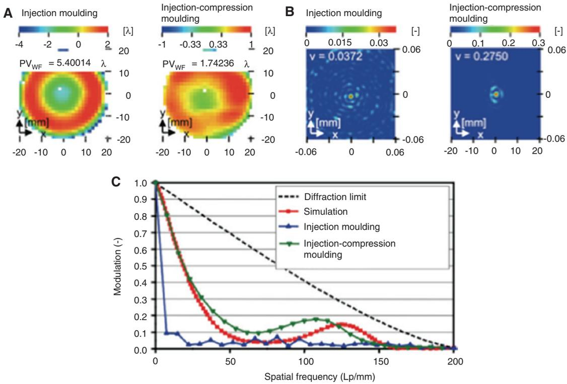
**Figure 22:** Injection molding and injection compression molding of lens: (A) measured deformation of the wave-front topography, (B) point spread function, and (C) modulation transfer function [40].
