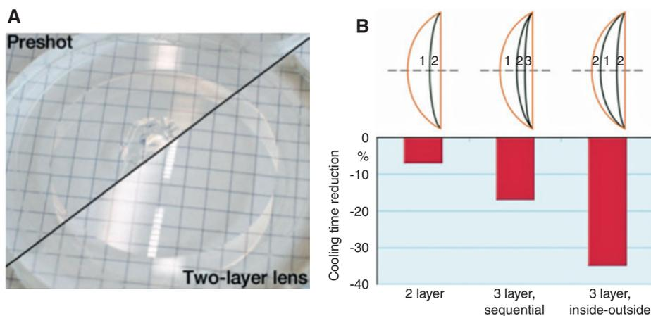
Figure 15: Multi-layer injection molded lens: (A) Preshot with surface defect before and after overmolding of a 2-mm-thick layer of plastic, (B) simulation results for various molding sequences: compared to the single-layer approach, the multi-layer process reduces the cooling time considerably. The cavity wall temperatures are color-coded [46].
