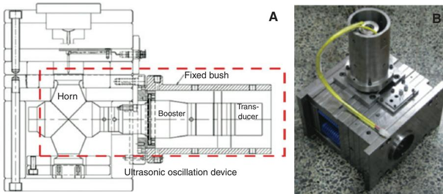
Figure 19: Ultrasonic assisted injection mold [58].
