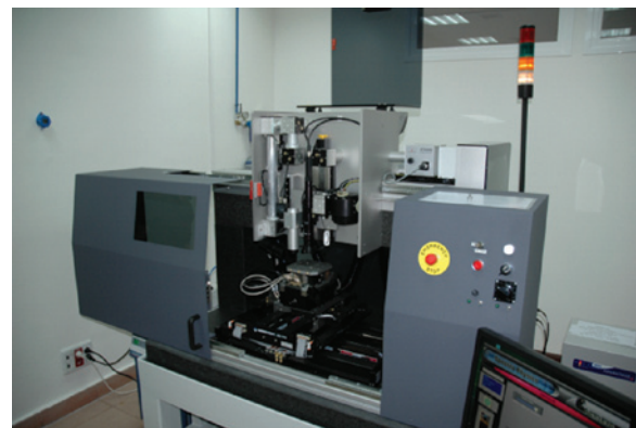
Figure 1: Experimental workstation equipped with ns pulse UV DPSS laser used for the reported experiments at UPM Laser Centre.
