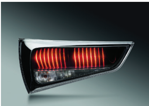
Figure 14: Hella styling sample of a rear lamp with special textile effect fabric.
