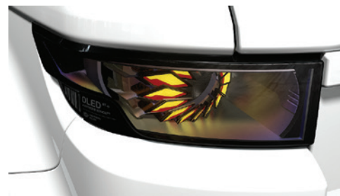
Figure 13: Hella styling sample with two-colored OLED.
