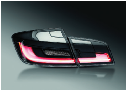
Figure 6: Hella styling sample EdgeLight, based on BMW 5series rear lamp.
