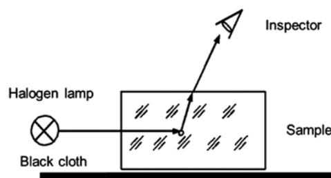
**Figure 4:** Inspection setup for bubbles and inclusions.
