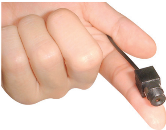
Figure 1: A pinhole lens.
