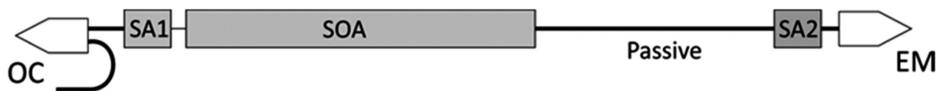
Figure 9: Sketch of linear passive mode-locked laser. Multimode interference reflectors (MIRs) with 50 and 100% reflection were used as mirrors. Three active sections (gray) were positioned in the way that colliding and anticolliding designs were realized. Figure from [21].
