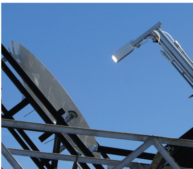
Figure 4 Example of a paraboloid and a central receiver test setup as installed at the Fraunhofer ISE [54]. Here, the diameter of the concentrating mirror is 1.2 m, while the receiver has an area of 4.5 \times 4.5 \text{ cm}^2 consisting of four single-junction monolithically interconnected modules (MIMs) [55].
