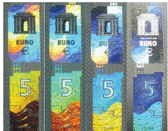
Figure 1 Diffractive structures on the €5 banknote. Four photographs were taken from a detail of the banknote. From one shot to the next, the incidence angle was changed so that different colors are perceived for the same areal position.
