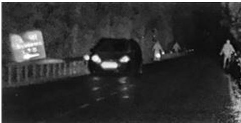
Figure 3 BrightEye™ raw imagery at night. Three dummy objects are noticeable (200 m, 150 m, and 100 m), a vehicle with low-beam headlamps at 75 m and a traffic sign (i.e., retro-reflector sign) is located 50 m from the AGIS.
