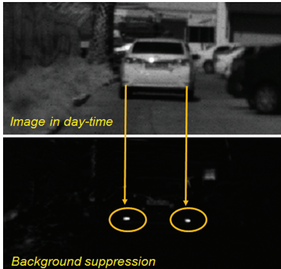
Figure 11 BrightEye™ retro-reflector detection during daytime.
