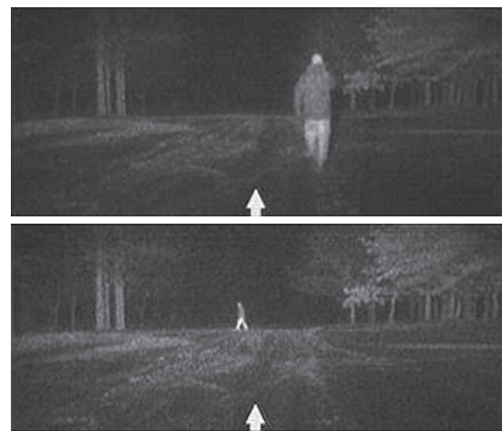
Figure 8 BrightEye™ imagery of a pedestrian between 50 m to 120 m during snow at night.
