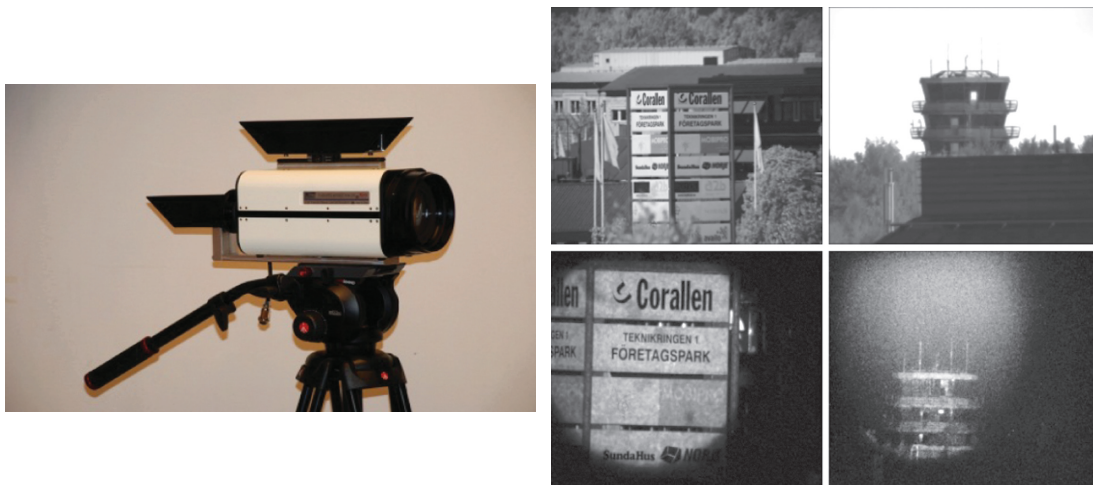
Figure 3 (Left) The camera (OWL SW1.7 CL 640) from Raptor Electronics including a telescope lens and a 1.5- \mu\text{m} , 1.6-W laser illuminator on the top. Images on the upper and lower rows show the passive (day time) and active images (during night), respectively. Range to the text board was 400 m and to the control tower, 2.5 km. Images FOI.
