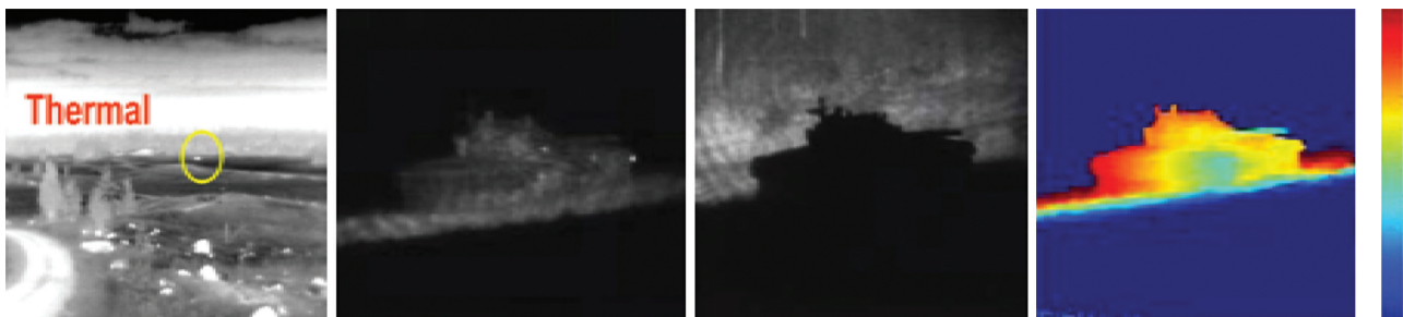
Figure 4 (Left) A potential target detected by a thermal imager. The next images show the target being observed by the range-gated laser system in the illumination, silhouette, and 3-D reconstruction mode. The range resolution is in the order of 20 cm despite the much lingered gate and pulse length. Images FOI, see Ref. [13].
