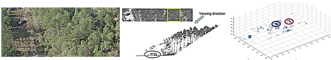
Figure 5 (Left) A part of vegetation with three vehicles, two of them occluded. The middle image shows an example of the power of 3-D ladars to see through vegetation. Above is the intensity image, and below is the 3-D image of the area within the square. The target (a tank) is encircled. The next shows all three vehicles visible (the occluded are encircled) and suitable for classification, for example, by template matching. Images FOI [35, 36].
