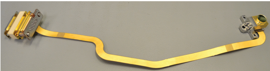
Figure 10 SLSTR detector with flex cable.
