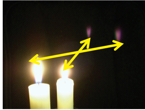
Figure 6 Picture of two candles with ghost images. The ghosts are reflections of the hot regions of the flame that are upside down. The picture was taken with a 6-megapixel DSC camera.
