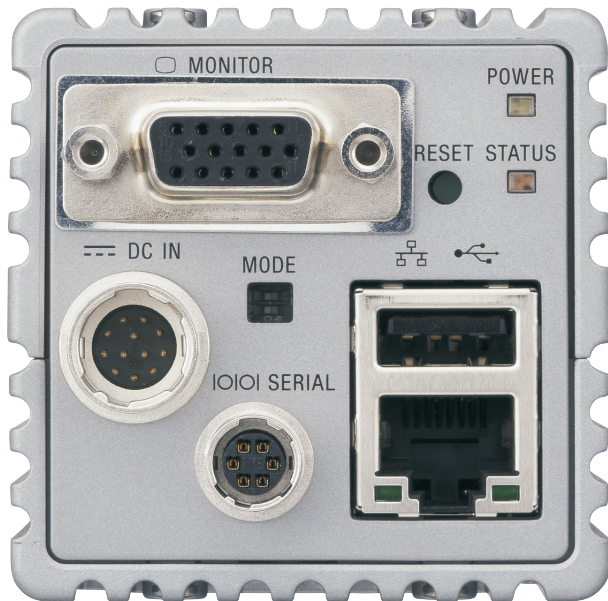
Figure 5 As the primary output of a smart camera is a decision or some type of signal other than an image, many smart cameras include integrated I/O and communication ports. This can include digital I/O, serial, Ethernet, and USB buses as well as display ports for user interfaces.
