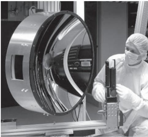
**Figure 7** LPP collector mirror.
