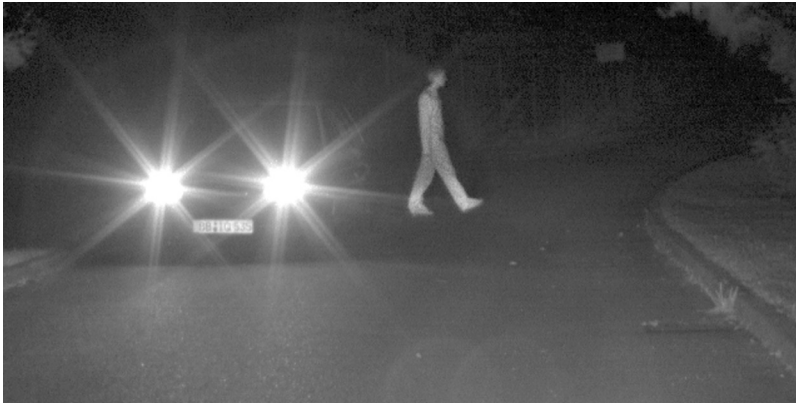
Figure 1 High dynamic range scene captured with a HDRC® image sensor in an automotive application with extreme brightness conditions.
