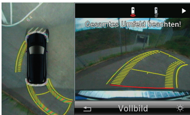
Figure 3 Mercedes-Benz GL-Class. The current state of the art is embodied by extended Active Parking Assist and the 360° camera on board the GL-Class. The surrounding area is visualized from different perspectives on the COMAND display, from a complete bird’s eye panorama to various detailed views which enable it to pinpoint maneuvering or reveal crossing traffic which is hidden in blind spots when moving out of narrow exits [12].
