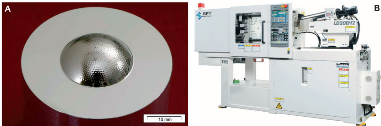
Figure 3 (A) Finished mold insert. (B) Sodick microinjection molding machine.
