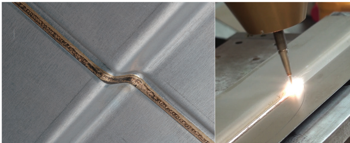
Figure 5 Brazing of fillet-weld lap joint (left) and flange weld joint (right).
