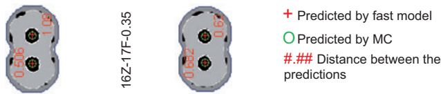
Figure 20 The accuracy of the fast 2D DSA model compared to 3D Monte Carlo model in the prediction of DSA via locations for merged guiding patterns [43].
