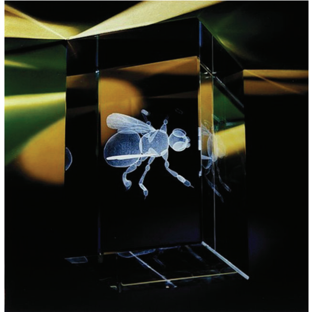
Figure 1 Three-dimensional image of a fly, sculptured in a block of glass. This image consists of more than 50 000 microcracks. Reproduced by friendly permission of the Institute for Laser Technology, Aachen (D).
