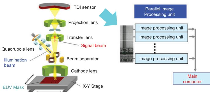
Figure 6 Basic configuration of the electron optics of the PEM and the parallel image processing system for the PMI.
