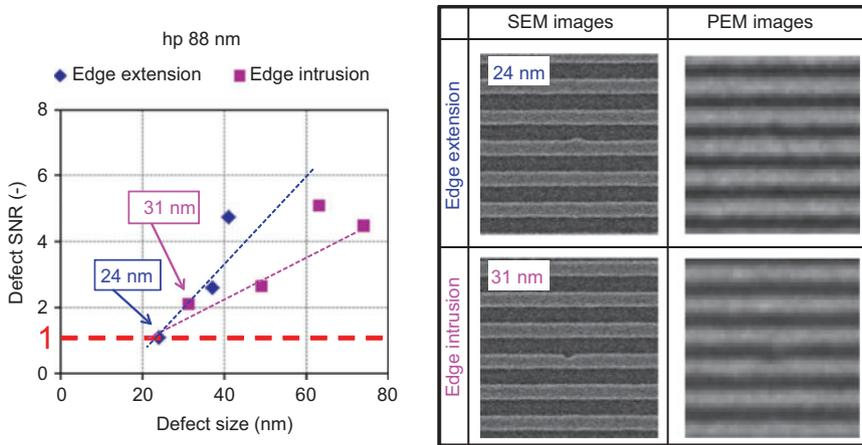
Figure 7 Preliminary test result for the SNR of the defect detection by the experimental setup.
