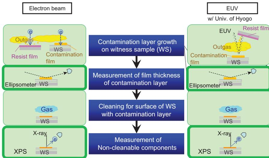
Figure 14 Resist outgassing qualification protocol based on the WS method.
