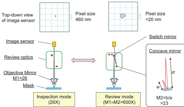
Figure 5 Schematic illustration for review optics of the ABI.
