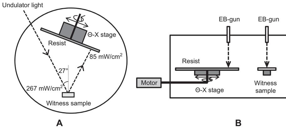
**Figure 15** Schematic representation of the outgas test setup, (A) HERC analysis tool, (B) EB-based resist contamination analysis tool, named the EUVOM-9000 (made by Litho Tech Japan).
