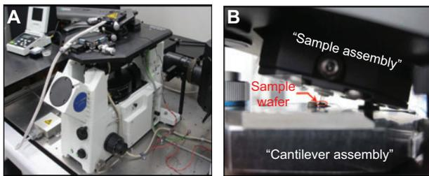
**Figure 11** Picture of the HS-AFM system (Nano Live Vision by the Research Institute of Biomolecule Metrology).
