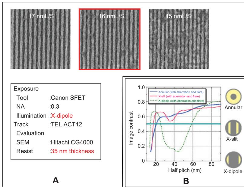
**Figure 10** Ultimate resolution of SFET utilizing x-pole illumination; (A) experimental result, (B) simulation on image contrast analysis.
