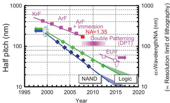
**Figure 1** Trend and prospect for downscaling of LSIs and lithography to be printed.
