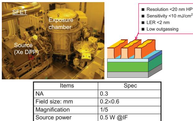
Figure 9 SFET and basic specification.
