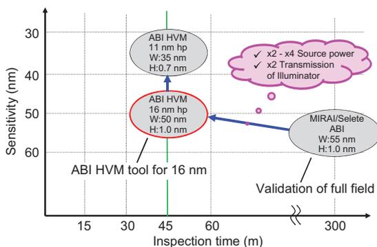
Figure 4 The progress of sensitivity and inspection time.
