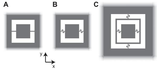
**Figure 12** Structural features of scanning micromirrors. A one-dimensional mirror with a torsion bar mount for movement in the  $y$  direction (A); one-dimensional mirror with a spring mount for movement in the  $y$  direction (B); and a dual-spring gimbal mount with a moving intermediate frame for two-dimensional movement in both the  $x$  and  $y$  directions (C). Not to scale.
