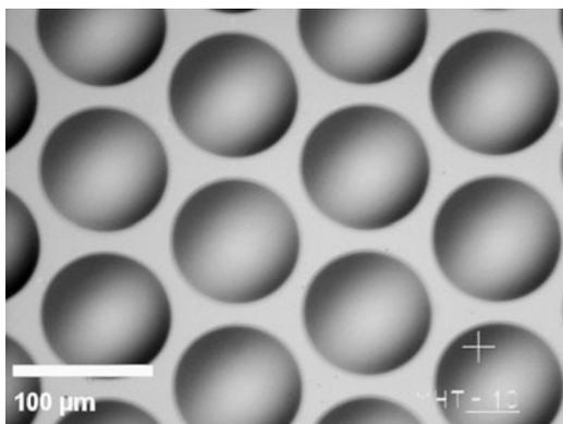
**Figure 3** Microcontact printed microlenses, formed in poly-alkyl-methacrylate; lens diameter is 90  $\mu\text{m}$ .
