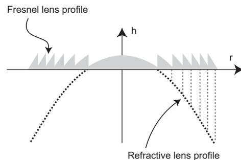
**Figure 8** How a Fresnel lens is assembled: the aspheric profile of the lens, shown in exaggerated form by the dotted line of the parabola, is folded upwards in discrete segments. Each segment retains the curvature of that part of the lens from which it was taken.
