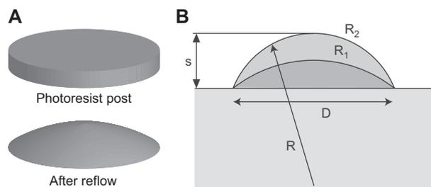
**Figure 1** (A, B) The high-temperature reflow of a cylindrical post of photoresist causes the cylinder to assume a hemispherical shape and thus a segment of a spherical lens.
