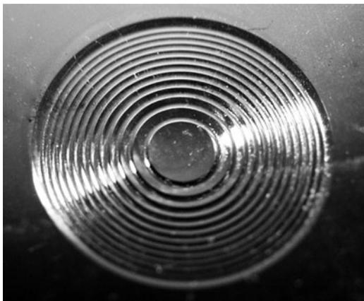
**Figure 9** A Fresnel microlens fabricated by embossing into PMMA; the lens has a diameter of 2.7 mm and a maximum sag height of 88  $\mu\text{m}$ .
