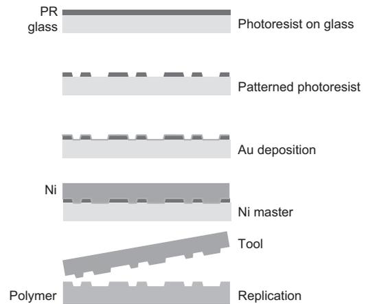
**Figure 4** Basics of replication: (top to bottom) photoresist on a substrate, typically glass; exposed pattern, binary or continuous relief; deposition of Au contact layer; electroplating a Ni master; replication in a polymer using the resultant molding tool.
