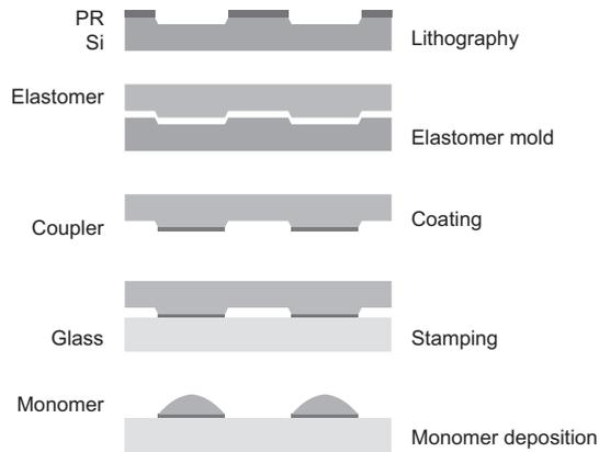
**Figure 2** Microcontact printing process for fabrication of self-assembled microlenses: (top to bottom) origination of a master in Si using standard lithography; molding the elastomer stamp; coating the stamp with a hydrophilic coupling agent; stamping on a glass substrate; lenses subsequently formed in a monomer by surface tension. Not to scale.
