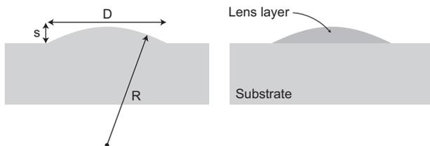
**Figure 6** Typical microlens structures, fabricated on a planar substrate; either the substrate material itself is patterned (left) or the lens is fabricated in a surface layer (right). The substrate is typically much thicker than the lens. The sag height is given by  $s$ , the aperture diameter by  $D$  and the radius of curvature by  $R$ .
