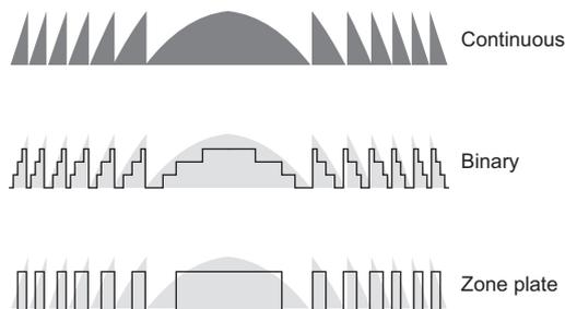
**Figure 11** The binary approximation of a continuous Fresnel lens profile (top) using a multilevel (center) or two-level (bottom) structure; the latter corresponds to a Fresnel zone plate.
