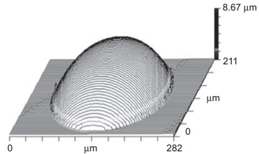
**Figure 7** The profile of a polymer microlens fabricated on a silicon substrate, measured using a white light interferometer. The sag height of the lens is approximately  $8 \mu\text{m}$ .
