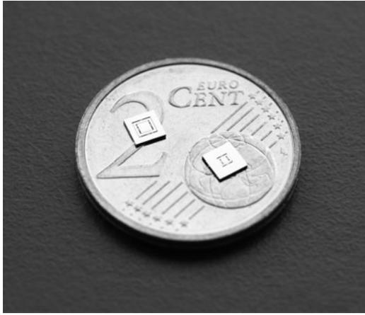
**Figure 14** Silicon-based two-dimensional scanning micromirrors on a 2-cent coin, with two differing mirror sizes. The chip sizes for both are  $3 \times 3$  mm.
