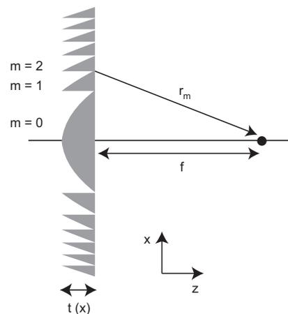
**Figure 10** Focusing an optical field using a Fresnel-like diffractive lens. The spacing between zone  $m$  and the focus  $f$  is an integral number of wavelengths longer than the focus,  $r_m = f + m\lambda_0$ .
