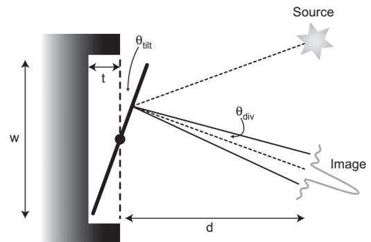
**Figure 13** Schematic cross-section of a tilting mirror used to image a point source; the dotted line from source to image denotes the path of the ray, but in reality an optical system would generate a (Gaussian) beam which comes to a focus at the image point. Dimensions and angles are not to scale.
