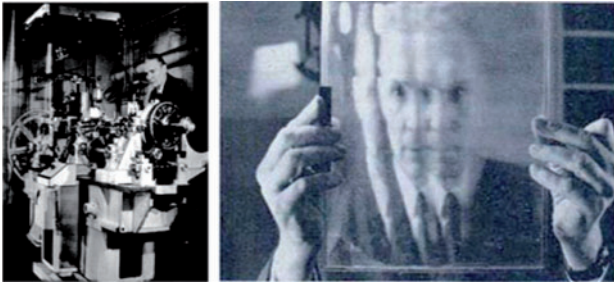
Figure 5 (Left) Maurice Bonnet and the lathe he used to engrave lenticular screens for integral photography, (right) holding one of his lenticular screens consisting of cylindrical microlenses [9].
