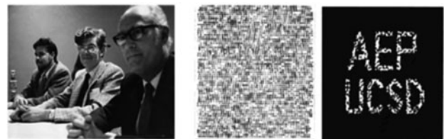
Figure 9 (Left) Photo of Adolf W. Lohmann with Byron Brown (left to him) and Ronald Kay (right to him) at IBM in San Jose, (center) computer-generated binary hologram and (right) its reconstruction using laser illumination (Photo: Adolf Lohmann, private collection).
