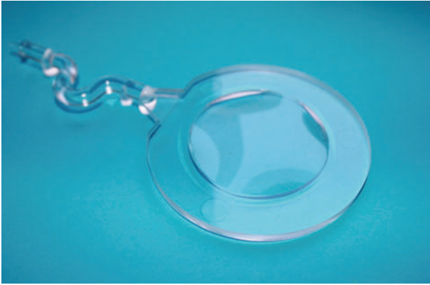
Figure 12 Molded freeform optical element with defined Zernike surface including gate.
