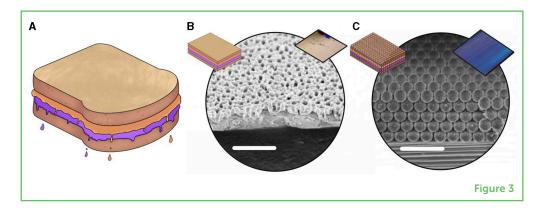
Once they master the basic recipe, scientists can experiment and create new ones. For example, they can make layers out of small, colorless glass particles—spherical objects that pack together and that have a similar size to the wavelength of visible light (Figure 3C).
