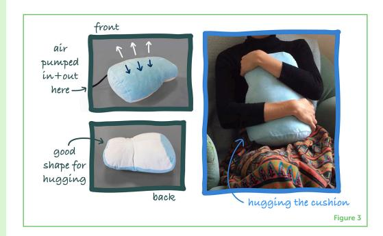
We made a robotic device that could push air in and out of a balloon inside the cushion, to control the "breathing". Because slower breathing is more relaxing, we used a slow breathing rate of 10 breaths per minute. Ten breaths per minute means breathing in slowly for 3 s and breathing out for 3 s—try it for a couple of breaths and see how you feel!
