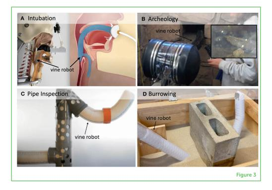
Vine robots have a lot of potential in the medical field. Figure 3A shows a vine robot being used to keep a person's airway open so the person can breathe, even if their airway is damaged or they are unconscious. Using the benefits of growing like plants, vine robots can squeeze through this gap and take the shape of the patient's airway, to safely and easily open it. Click here to watch a video of this vine robot in action.
