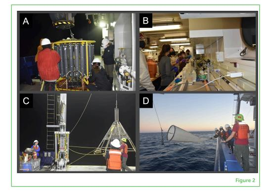
The water samplers are bottles that can be opened and closed deep in the ocean using electronics on the ship. The water samples allow us to measure what makes up ocean water and what lives in it. By filtering the water, we can look at particles of dust, DNA and nutrients (Figure 2B). Just for fun, we decorated styrofoam and sent it down to the deep ocean on the CTD! The weight of the ocean above it squeezed all of the air out of the styrofoam and made it a lot smaller (Figures 3A,B).
