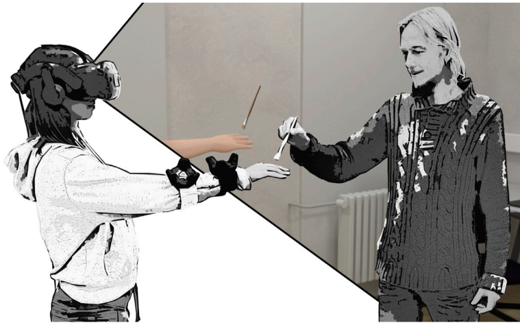
FIGURE 3 | Example of a virtual RHI setup. The black and white area depicts the participant (left) and experimenter (right) situated in the real environment. The coloured area represents the virtual environment, which the participant perceives via an HMD. When the experimenter stimulates the participant's real hand with a brush, the participant sees these brush strokes on a virtual hand in VR. The virtual hand model was taken from turbosquid.com under their standard license.
