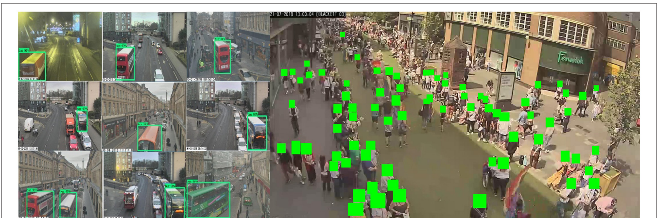
FIGURE 2 | Examples of bus counting and pedestrian flow monitoring using CCTV and machine learning from Urban Observatory sensors.
