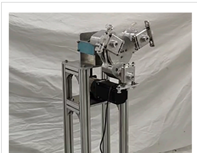
FIGURE 12 Cam-elliptical gear combination vegetables curved surface labeling mechanism.
