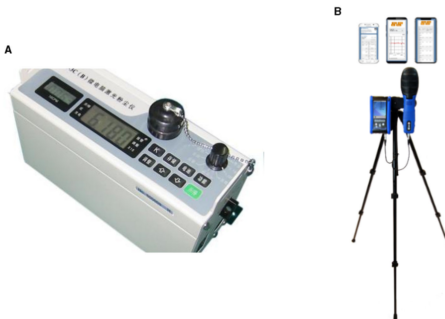
FIGURE 2 The adopted monitoring devices. (A) Laser dust meter LD-3C (B); (B) Multifunctional portable environmental quality inspection system instrument.
