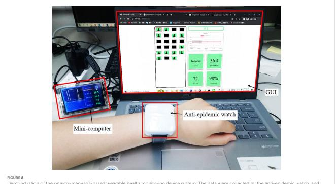
Demonstration of the one-to-many IoT-based wearable health monitoring device system. The data were collected by the anti-epidemic watch, and the mini-computer received the data and then uploaded it to the cloud server and database. The terminal webpage requested the data from a specific user and displayed it in real time. The demonstration is recorded in Supplementary Video S1.
